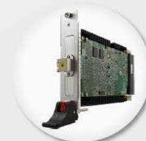
Air-Cooled VPX w/ Front Panel IO
