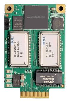
Alta continues to fill out the NLINE product family as interface cards are still the bread and butter of the COTS market. ARINC and 1553 network interface cards (NICs) are still very popular for embedded integration and test of avionics systems. Alta started with PMC, PCI Express, XMC, PXI style interface boards and then invented their ENET real-time Ethernet converter appliances, which became one of the
