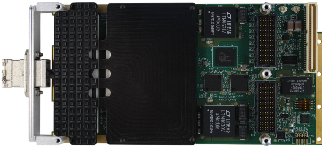
Figure 1: The V1153 is a rugged XMC FPGA card for high-speed interface and coprocessing solutions. It offers 4 to 12 optical port options (front panel or backplane) as well as 1-16Gbs electrical backplane ports.
