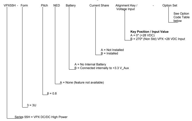
**Example:** VPX55H-38AABA-00 = 3U VPX DC/DC Converter; 0.8" pitch; no NED feature; no internal battery; current share on VS1, VS2, and VS3; +28 VDC innput; 500-Watt output power
