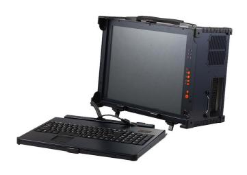
that prohibit the use regular laptops or less rugged lunchbox style computers. It has features that include removable hard drives, shock absorbing bumpers, a large LCD protected by a shatter resistant glass, NEMA 4/12 compliant keyboard pointing devices, dual cooling fans - all enclosed in a machined black anodized aluminum chassis.
