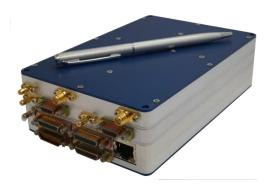
for Combined or Independent channel data demodulation from RF or IF signals. Digital multi-mode demodulation options include Multi-Symbol PCM/FM, SOQPSK, BPSK, QPSK, OQPSK, SQPSK, AQPSK, AUQPSK, PCM/PM, and Multi-H CPM. Analog FM demod is an option. Sub-carrier(s) demodulation can also be provided, other formats available upon request.
