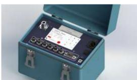
portable, battery powered, multi-mode test transmitter with an on-board PCM data source. The on-board PCM source is capable of providing IRIG PCM frame formats as well and PRN patterns, with and without injected errors. The unit is also capable of accepting external clock and data sources for test modulation, by-passing the on-board PCM generation source.
