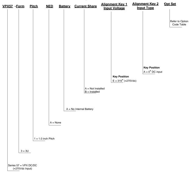
Example Part Number: |VPX57-31AABEA-00; 3U VPX DC/DC Power Supply, 1.0" pitch, current share on VS1, VS2 and VS3, +270Vdc Input, no additional options
